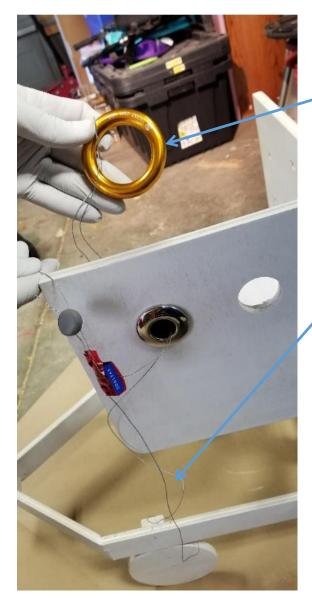
Ring allows wire to be mounted through the hull, avoiding removable locations
