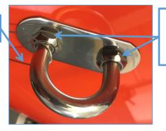
Two nuts (front and backside) easily removed, allowing disconnection from boat
